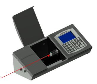
1. Place cell in right hand side of sample chamber
