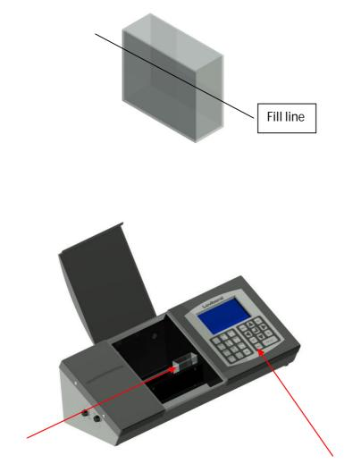
1. Place cell in right hand side of sample chamber. 2. Press [ZERO]
