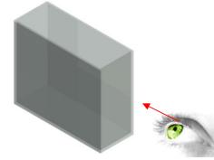
Completely clean the measurement cell before use. Any residual marks from the packaging wrap will result in a failed calibration.Check cleanliness by looking down the light path.
